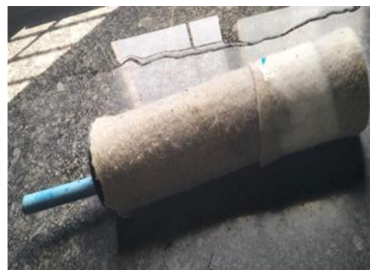
Fig 5.5: Geo composite Salt Barrier
